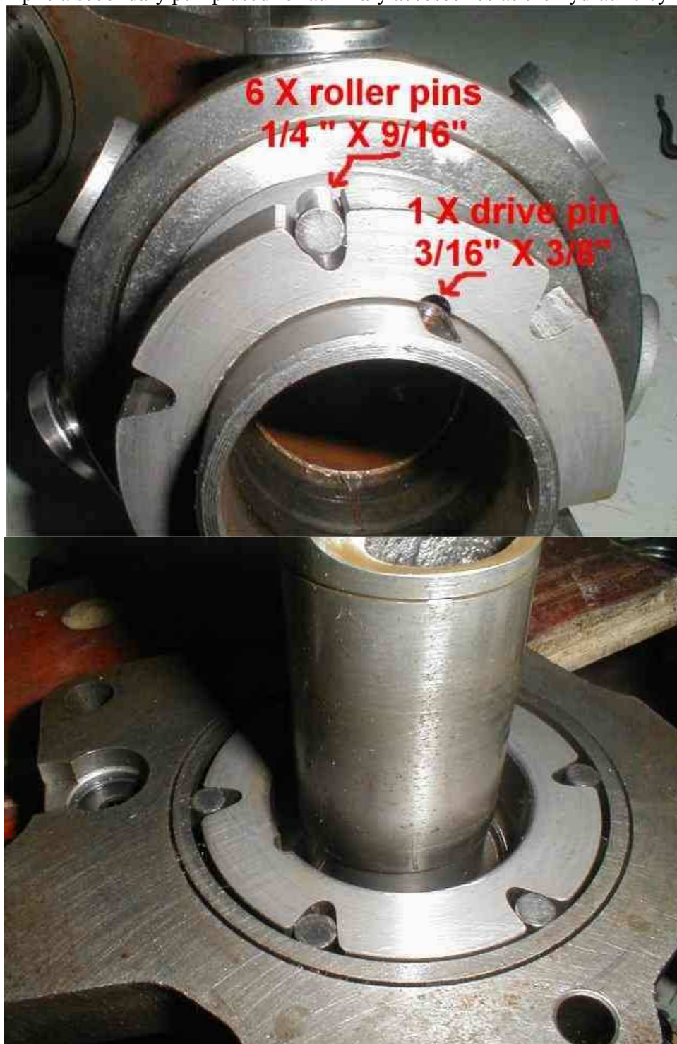
Six rollers pins 1/4 X 9/16
